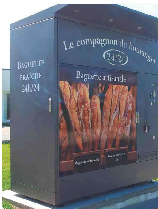
The Compagnon du boulanger vending machine includes an oven to finish off prebaked baguettes.
