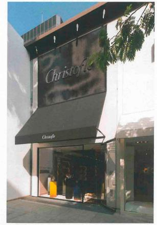
Above The storefront's shimmering signage was custom made with 4000 metal pins.
